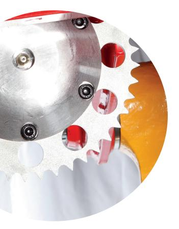
**The length measuring unit** is actuated by an extremely well protected hydraulic cylinder and encapsulated hoses, enabling the measuring wheel to be retracted into a protected position when the head is opened.
